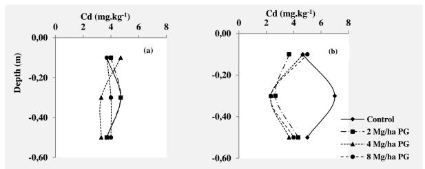
**Figure 4.** Trends in soil Cd content (mg.kg<sup>-1</sup>) by Depth, of Nefza acidic soil under crock oak forest amended with PG as surface application (a) and with mixing of PG (b)
