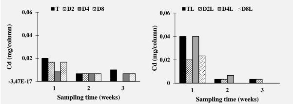
**Figure 1.** Cadmium amount in leached solutions for the different treatments. T, D and DL denote control, phosphogypsum rate and mixture of litter and phosphogypsum. 2, 4 and 8 denote the PG rates of 2, 4 and 8 t PG.ha<sup>-1</sup>, respectively.
