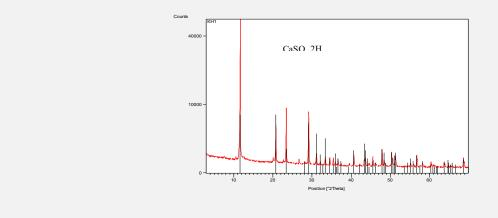
Figure 1. X-Ray Diffractogram of powdered PG ( $\Box \Box Cu$ =1.54 Å)
