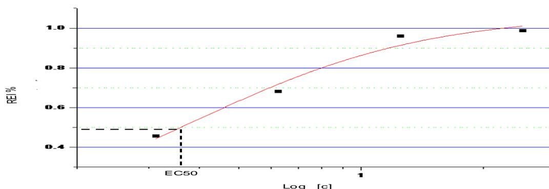
**Figure 1:** Graphic determination of the effective concentration of sewage sludge that inhibits the root elongation (REI) lettuce seed by 50% ( $\text{EC}_{50}$ ) with respect to inert sand. [C] represents the % concentration of sludge in the mixture sludge-sand.
