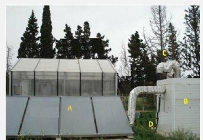
**Figure 4:** shows a diagram of the experimental system. This unit includes:,(A, C, D) solar panels and a fan, inducing the processes of air humidification (evaporation) and dehumidification of the air (condensation), a storage tank (B) (Chouaieb, 2007).
